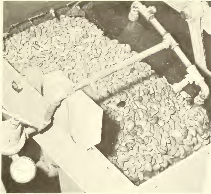
Figure 1.--Apparatus for spraying almonds with malathion EL.
